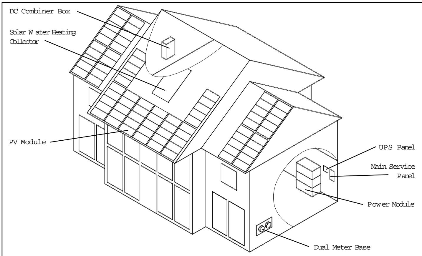
Figure 2. The NCSU Solar House PV System.
