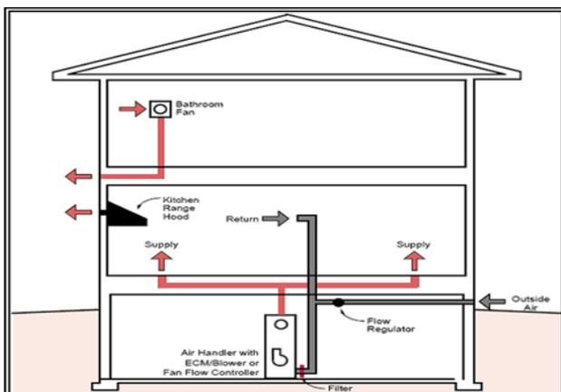
Fig. 2: Spot ventilation & HVAC integrated supply
