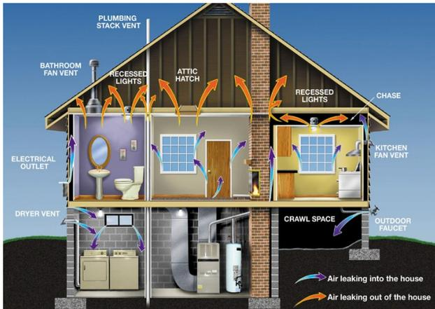
Fig. 1: Common building envelope air leakage sites
