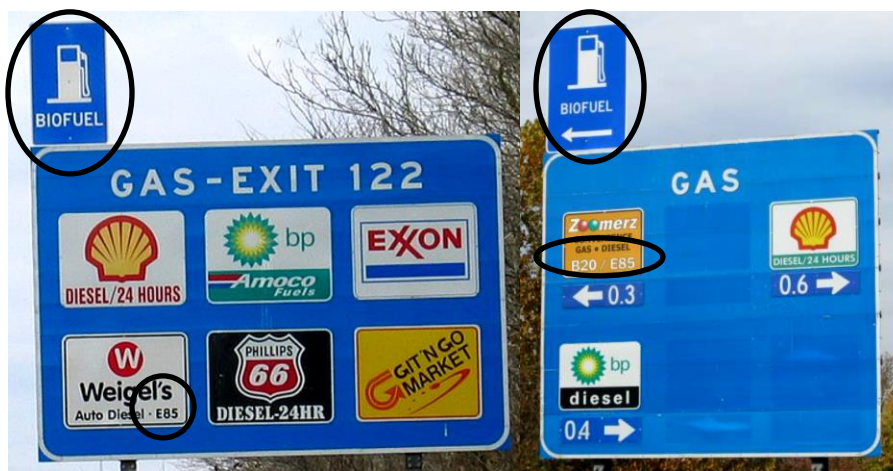
Figure 5. Left: Logo sign on the interstate (no arrow), note that the Weigels logo has E85 as supplemental text. Right: Logo sign on the exit ramp (arrow included), note that the Zoomerz sign has B20 and E85 as supplemental text.
