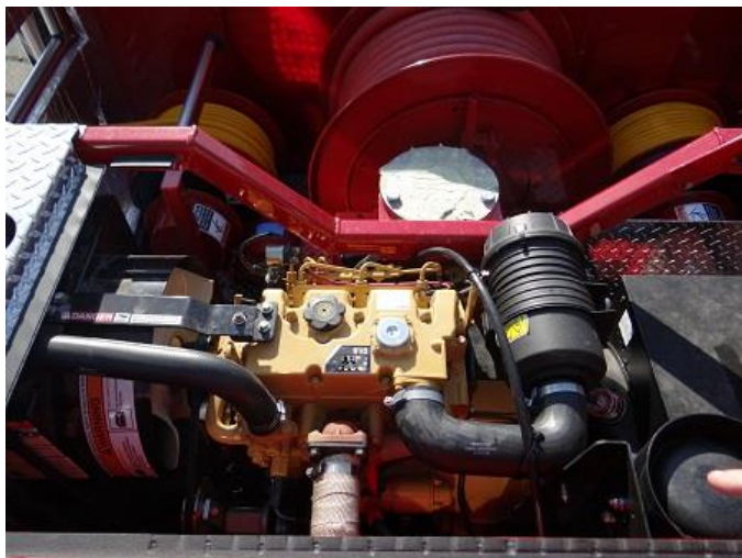
An Auxiliary Power Unit (APU) found in one of the fire trucks operated by the City of Charlotte Fire Department. Photo by Power2Charlotte
