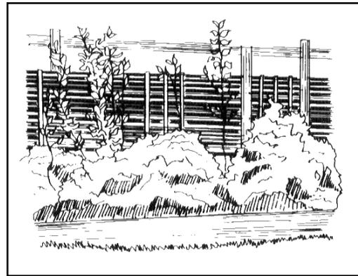
*Figure 8. Vines on a trellis can provide effective summer shading. Keep them several inches away from the house to avoid moisture build-up.*
