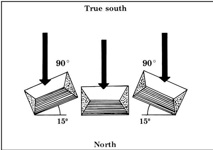
**Figure 2.** The south-facing wall can vary up to 15° either east or west of true south and still be effective for solar collection.
