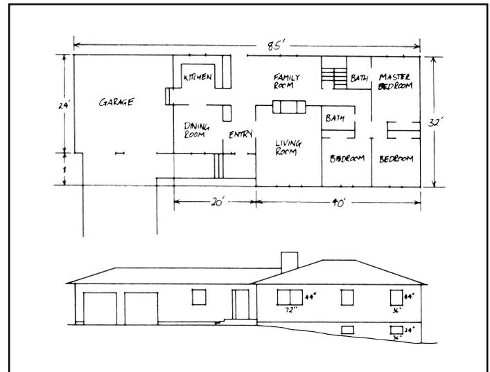
**Figure 1. Sketch the floor plan of your house, noting dimensions, window locations and the south facing wall.**
