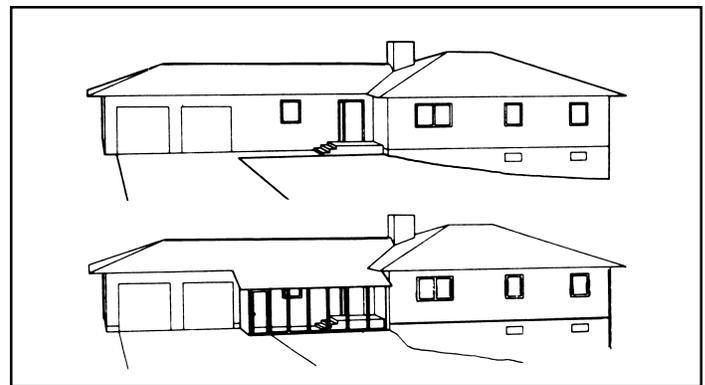
**Figure 8.** The sunspace or attached greenhouse is usually the most expensive passive solar retrofit, but it can provide the most supplemental heat. You should be able to close off the sunspace from the rest of the house.
