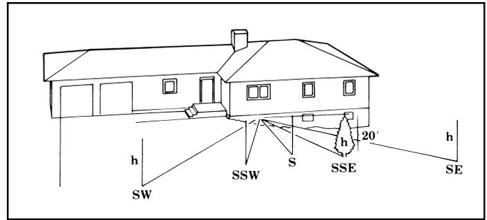
**Figure 3.** Solar access can be evaluated by the amount of shading on the south wall. For example, a 20 foot evergreen to the south-southeast of the reference point needs to be 36 feet or further from the south wall to avoid shading it.
