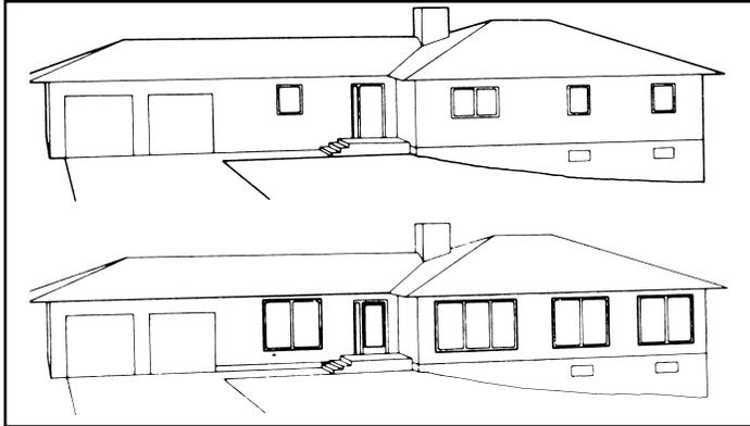
**Figure 4.** A direct gain system may be the easiest and least expensive passive solar retrofit. Extra mass is not needed if south windows are less than 7 percent of the floor area.
