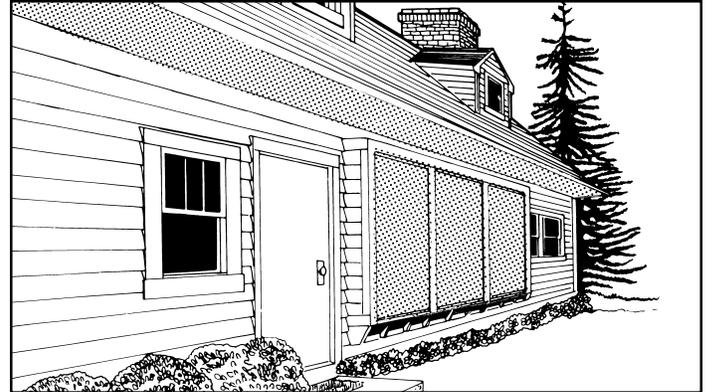
**Figure 5.** A thermosiphoning air panel (TAP) can be used when it is impractical to add windows to a south wall. Air that is heated in the collector panel circulates to the living space through vent openings.
