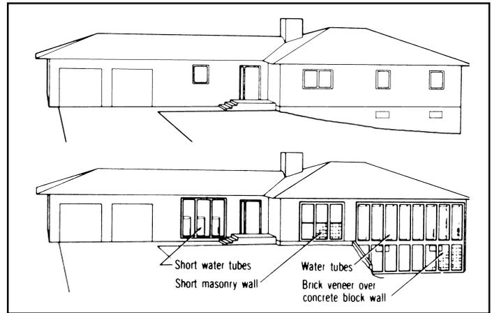
**Figure 7.** A Trombé wall uses mass placed very close to the south-facing glass. It may cost more and perform less efficiently than a direct gain retrofit.
