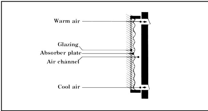
**Figure 6.** To prevent reverse cycling of air flow at night, and to keep heated air out in the summer, the TAP should have dampers.
